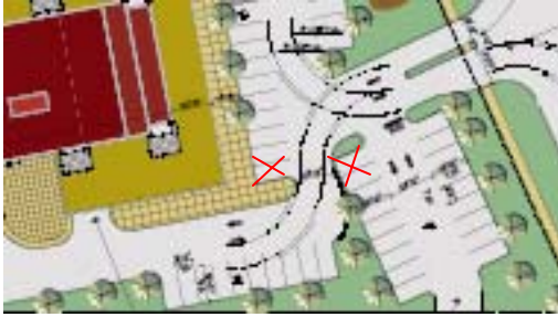
Circulation to retail loading dock is circuitous and could block main entry to site.
