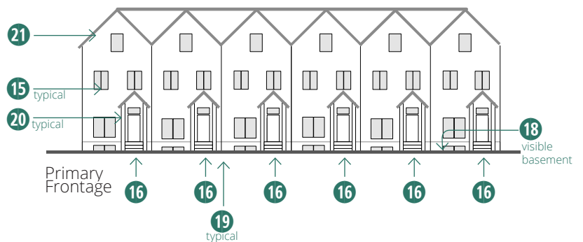
Figure 11-6(15) Row Building: Facade Design Requirements
